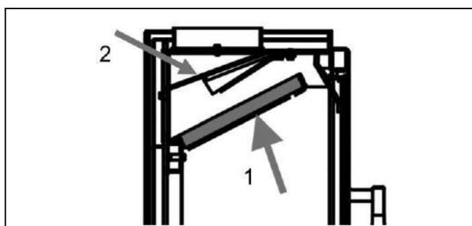
To sweep the flue, remove the vermiculite baffle (part 1) and unscrew the baffle plate (part 2). After sweeping away the soot and cleaning, proceed in the reverse order to reassemble the unit.
